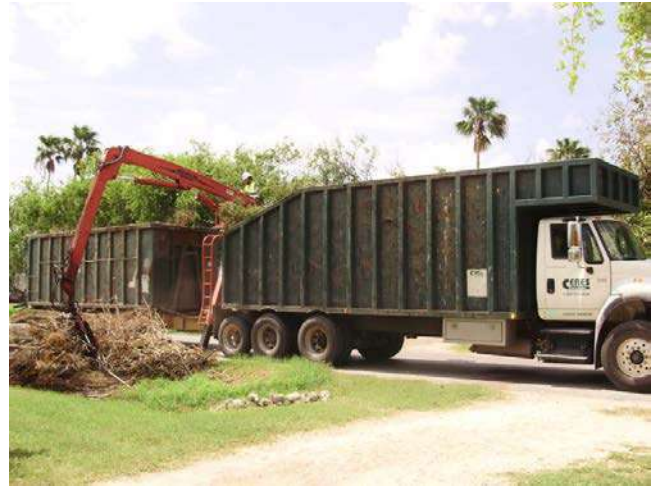
A Ceres self-loader with a trailer making pickups from the ROW.
